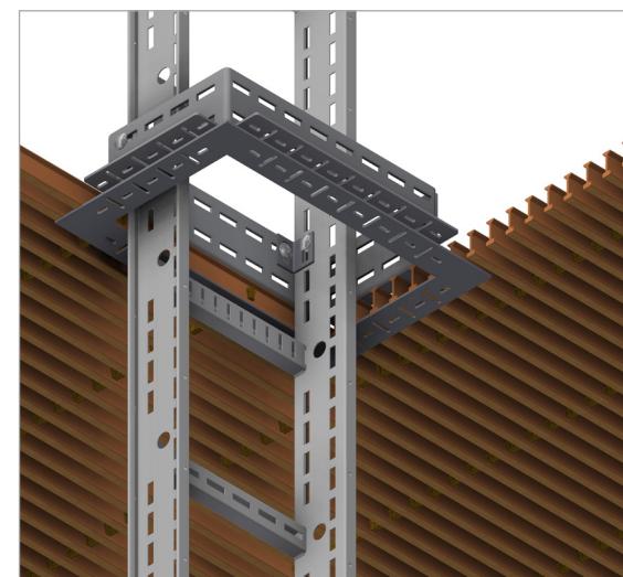
Ladder is attached using OE angle brackets.
