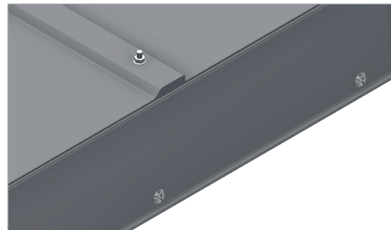
1. The cover is supplied with fasteners and the clamps can be fitted after assembly.
