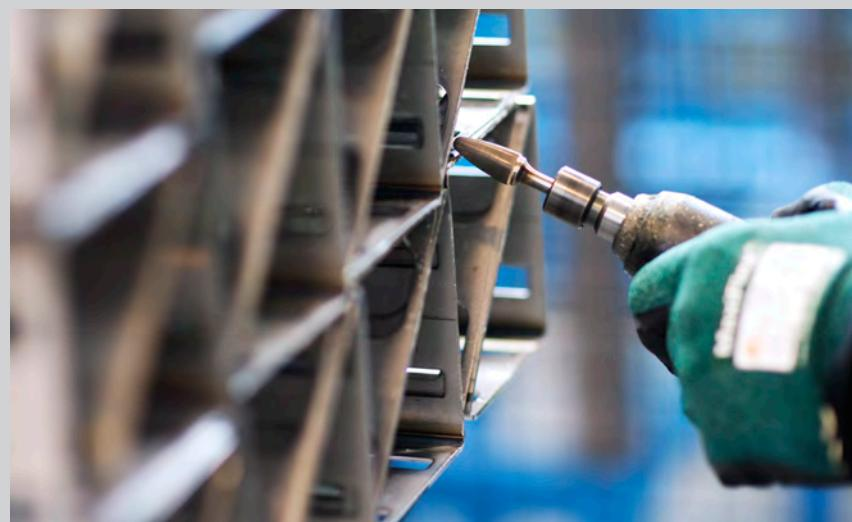
After metal has been cut, all sharp edges should be deburred to avoid cutting injuries to personnel.
