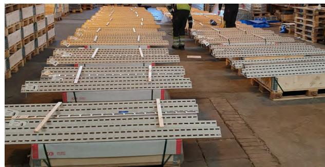
bulk. All assemblies are carefully wrapped to protect the material from site contaminants and damage due to weld splatter, paint and other such contaminants at the site.
