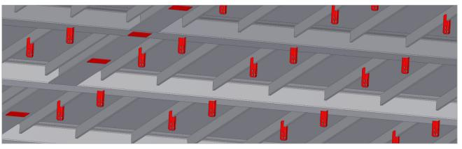
Oglaend MultiGrid® System, combining welded starter brackets for beams and stringers.
