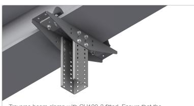
Traverse beam clamp with CH100-3 fitted. Ensure that the reinforcing plate is fitted so the width matches the top clamp.
