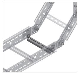
**Typical application:** Extra rung to support cable on transition to flexi-riser. Single fixing enables the rung to be rotated to the ideal angle to support the cable.
