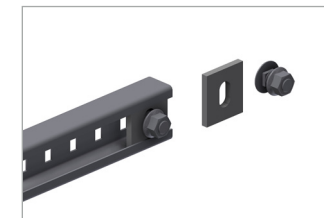
Bolt the back rungs on the inside of the rack sides using washers.
