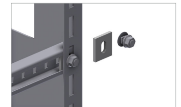
Bolt the back rungs on the inside of the rack sides using washers.
