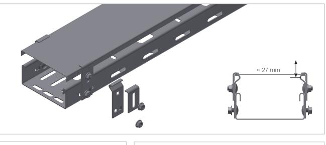
Clamps for SPB-RF100 have extra holes for fixing.
