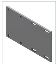
For expansion couplers, place one coupler at approx 25 m intervals to mediate thermal expansion for temperature variations of  $\pm$  20 °C.
