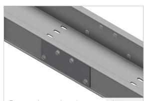
For expansion couplers, place one coupler at approx 25 m intervals to mediate thermal expansion for temperature variations of  $\pm$  20 °C. Thermal expansion coefficient: 25x10-6 mm/mm °C.
