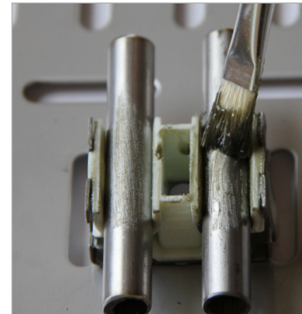
Step 2: Place the tubing in the clamp and apply CPP on the contact area between the tubing and the cover.
