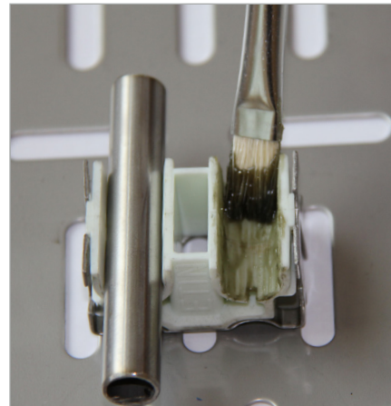
Step 1: Apply the CPP on the surfaces directly in contact with the tubing.
